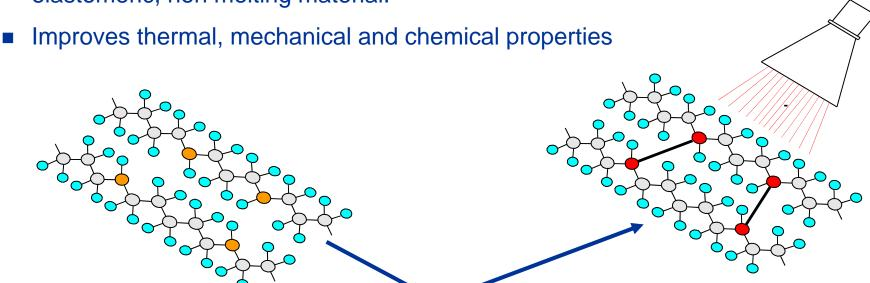
Thermoplastic material transforms into elastomeric structure
